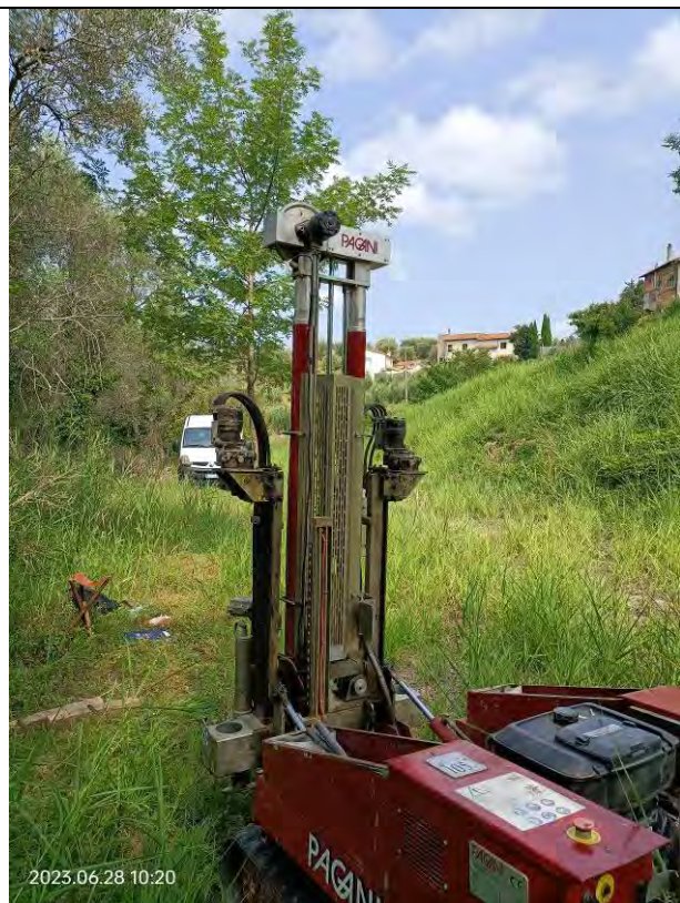
Penetrometria P4 (DPSH)
