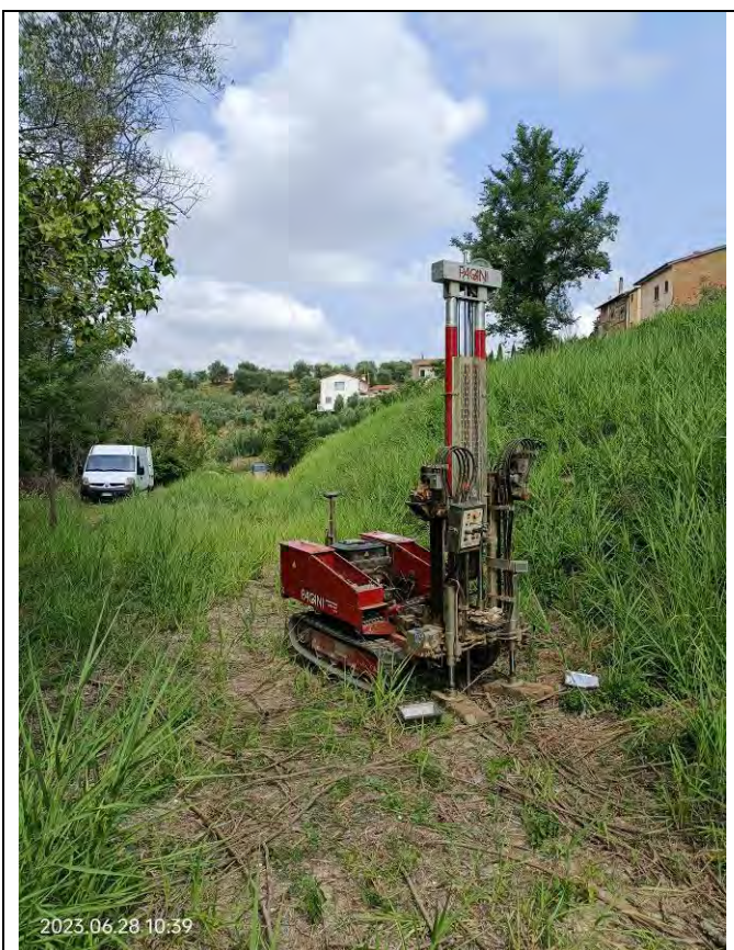
Penetrometria P5 (DPSH)
