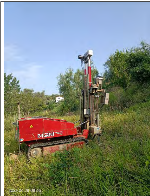
Penetrometria P3 (DPSH)
